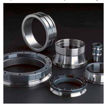
precision that currently be achieved with hard turning", and he backs up his statement with numbers: "With these machines, the following tolerances can be achieved on work pieces having hardness of up to 70 HRC and up to a diameter of 1500 mm: a surface accuracy of Ra = 0.0001 to 0.0004 mm, shape accuracies between 0.0002 and 0.001 mm as well as dimensional accuracy of 0.002 mm or smaller."
